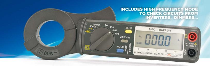
The CT-237 is a precision AC clamp digital measurement instrument to measure leakage currents, including operating mode selection for low frequency (50/60 Hz) or high frequency (up to 1 kHz). Both under numerical mode and 20 samples per second bar graph. Includes a filtering circuit designed to get rid of the high frequency parasitic noise and the harmonics for AC currents measurement.
